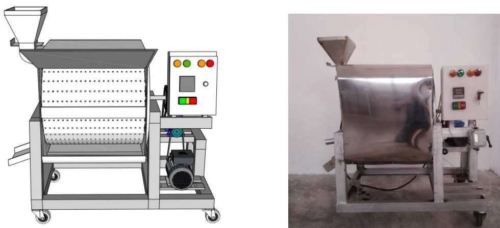
Figure 1. Electric heat source roaster with a power of 1800 watts.
