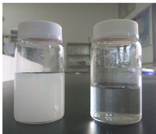
Figure 9. Comparison of the sample solutions before and after filtration by the PVDF1 membrane.
